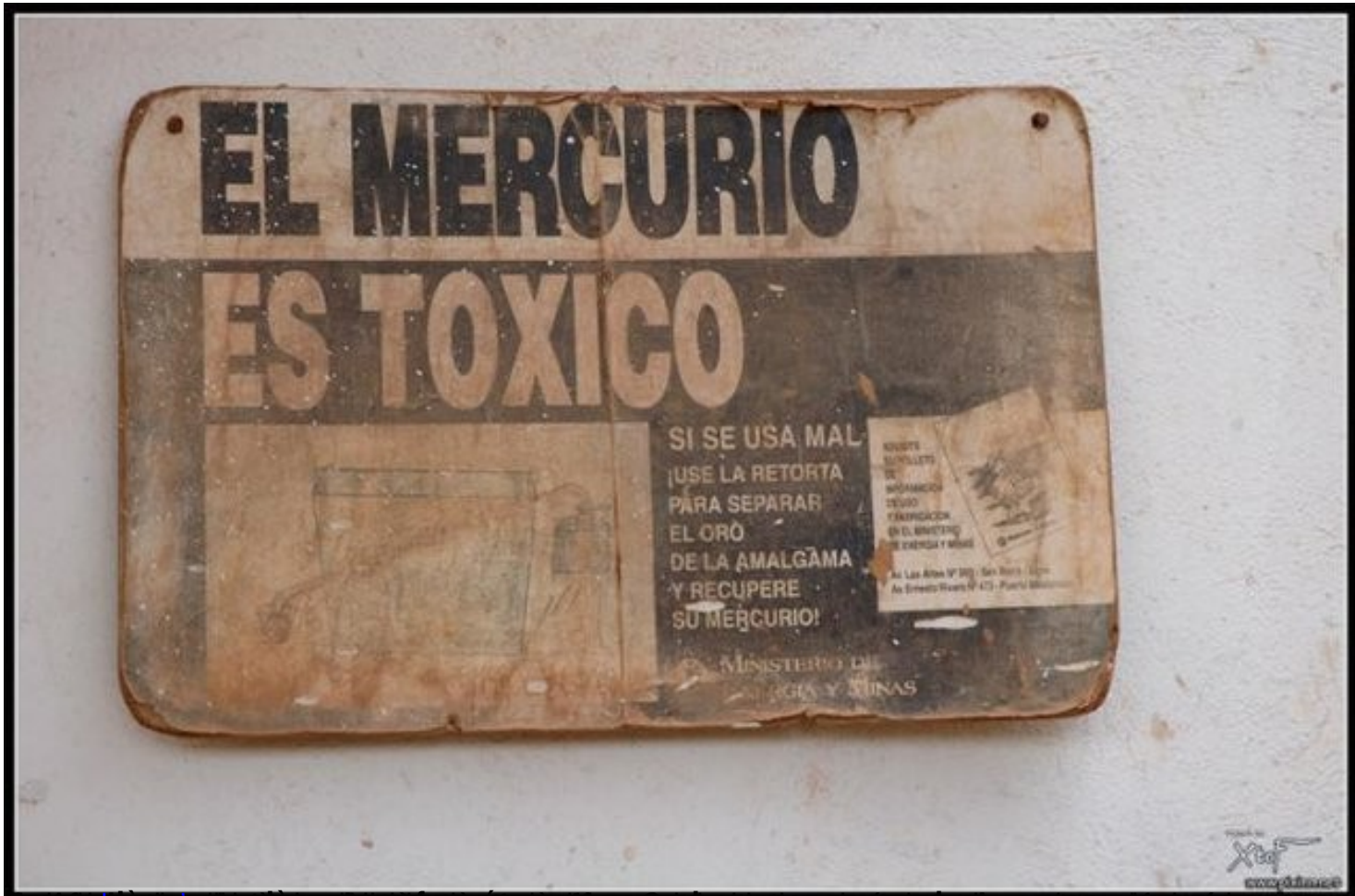
Historical poster on the toxicity of mercury and the use of retorts to separate gold from amalgam and recover the mercury.
